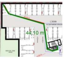
4. Travel via fireisolated exits The path of discharge from the Eastern fire stair currently occurs within 6m of the external opening serving the entry lobby which are not proposed to be protected by a method listed within BCA Clause C3.4
